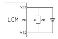
$V_{\text{DD}} \sim V_0$ : LCD Driving voltage
